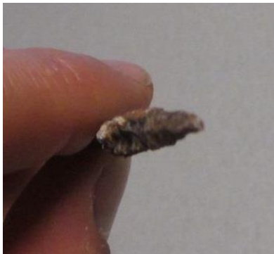
Figure 11: East Gymnasium Wall, Ladder Type Wire Joint Reinforcement Corrosion
