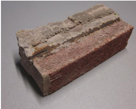
Brick with Corroded Joint Reinforcement
