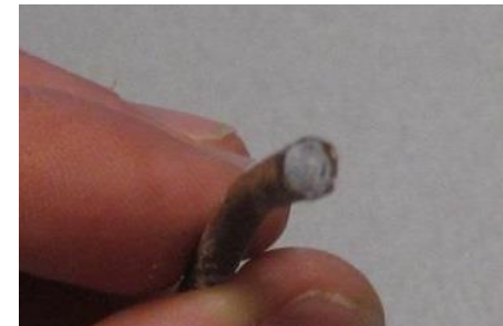
Figure 6: South Wall, First Floor Ladder Type Wire Joint Reinforcement Section
