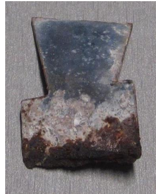
Figure 9: East Gymnasium Wall, Dovetail Wall Tie Corrosion
